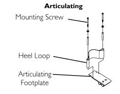
FIGURE 6.12 Composite/Articulating Footplate Heel Loop Replacement
